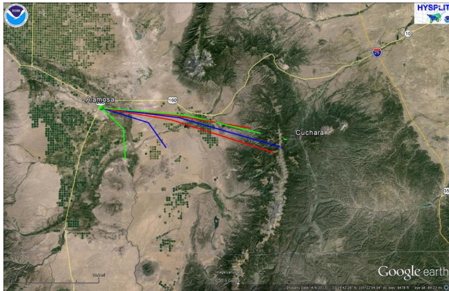
Figure 20: NOAA HYSPLIT 12 km NAM 2-hour back trajectories for Alamosa, CO from 5:00 PM MST (0Z June 21) June 20, 2012, to 11:00 PM MST (6Z June 21) June 20, 2012. (Source: http://ready.arl.noaa.gov/HYSPLIT.php )
